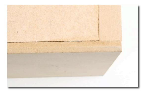
As you can see in the photo above, gaps in the joins can also be present due to inadequate pressure during the construction process. These should also be filled using a spackle filler. Please note that many fillers are not suitable for use with DuraTex. Be sure to use a spackle type filler (shown below). Make sure you also observe the drying times on the filler you are using before proceeding.
