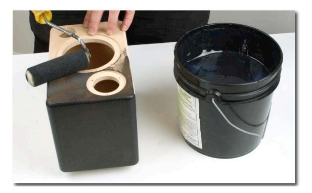
As an example only of thick application, here the back receives a thick coat (image 9). Thicker application can mean less coats are required but this also leads to a heavier texture and is not ideal near recesses, particularly on the front baffle.
